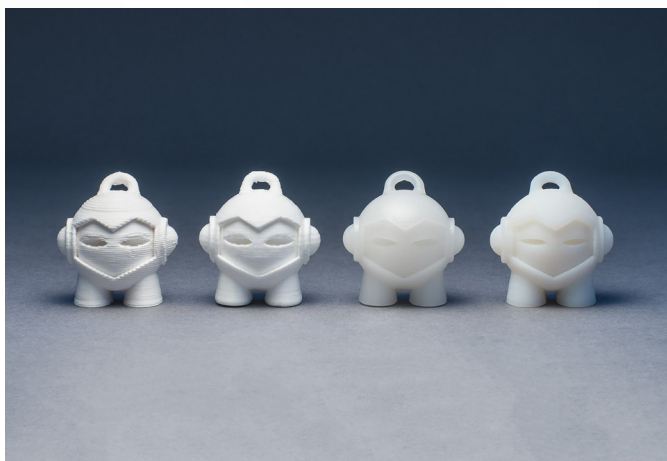
Figure 5.2. Marvin printed in 200 microns FDM, 100 microns FDM, SLA and Material Jetting (from left to right) Source: www..3dhubs.com
