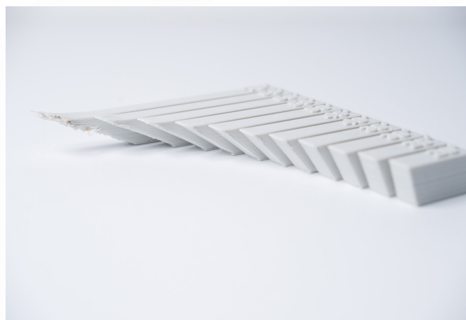
Figure 5.1. The effect of increasing angle on overhang quality for FDM printing Source: www..3dhubs.com
