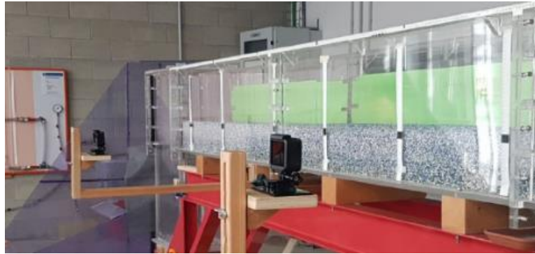
Figure 2-27 Cameras positioned in front of the channel
