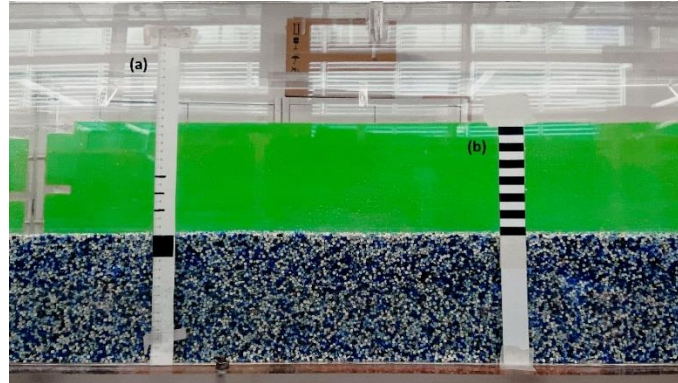
Figure 2-3 Installed rulers on the wall of the channel used as an indicator for the bed elevation (15 cm) at the initial stage of the experiment and as a tool for validation
