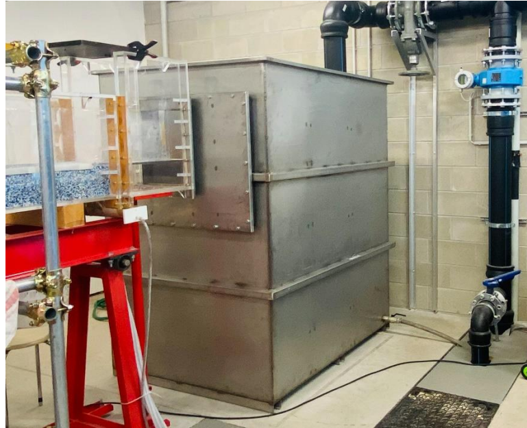
Figure 2-7 Upstream water tank
