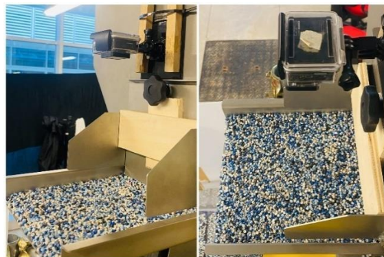
Figure 2-13 The camera used for recording the sediment movement along the vibrating channel
