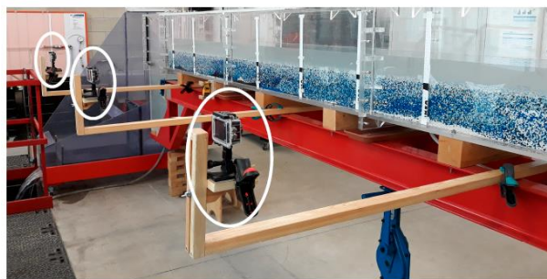
Figure 1-5 Cameras for measurement of bed elevation (Radice et al. 2018)
