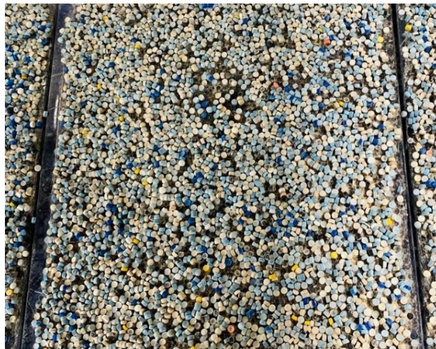
Figure 2-4 Plastic plates located in the first 75 cm of the channel
