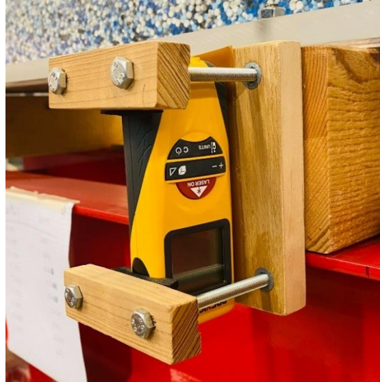
Figure 2-5 Laser distance meter fixed to the channel
