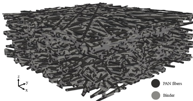
Figure 4.1 Result of the geometry generation algorithm. A three-dimensional sample of a gas diffusion layer made by carbon fibers (black colored) and binder (gray colored).
