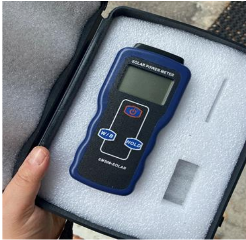
Figure 28: Solar Power Meter SM 206- SOLAR
