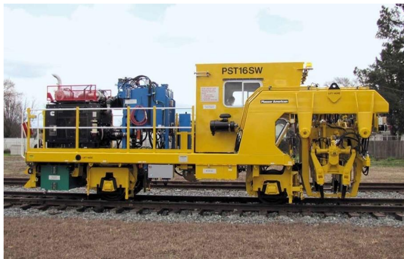
Figure 15. Tamping machine. (The constructor, 2019).
