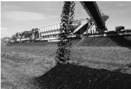
Figure 18. The undercutting operation (Li, Hyslip, Sussmann, & Chrismer, 2015).
