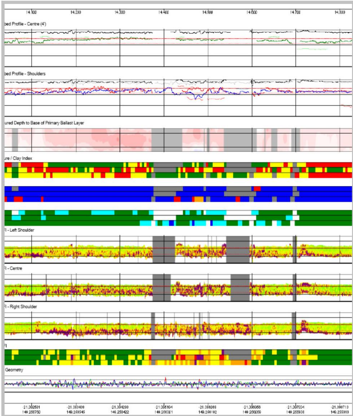
Figure 38. Report with data panels showing (top-bottom) – layers in the center, layers over the shoulders, a contoured map of depth to fouled ballast/formation, colour strip charts showing moisture index, thickness of ballast against defined thresholds, and ballast layer roughness, 2D BFI plots, colour strip charts of the 1D BFI, and track geometry (Top Up and Down + Twist). Linear meterage and GPS coordinates provided. (Eriksen, Gascoyne, & Fraser, 2011)
