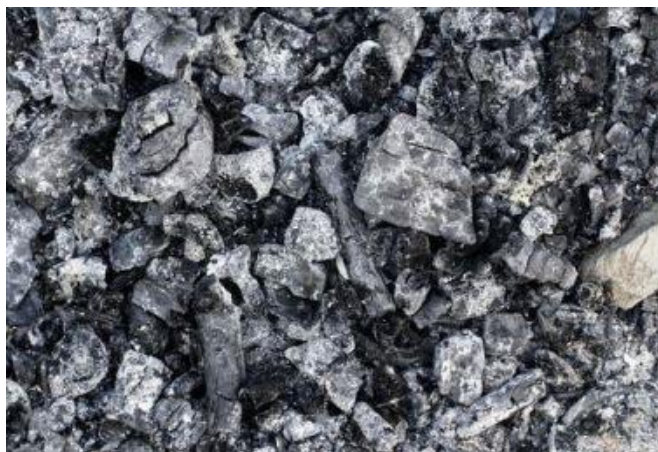
Figure 4. Coal ash ballast. (The constructor, 2019).
