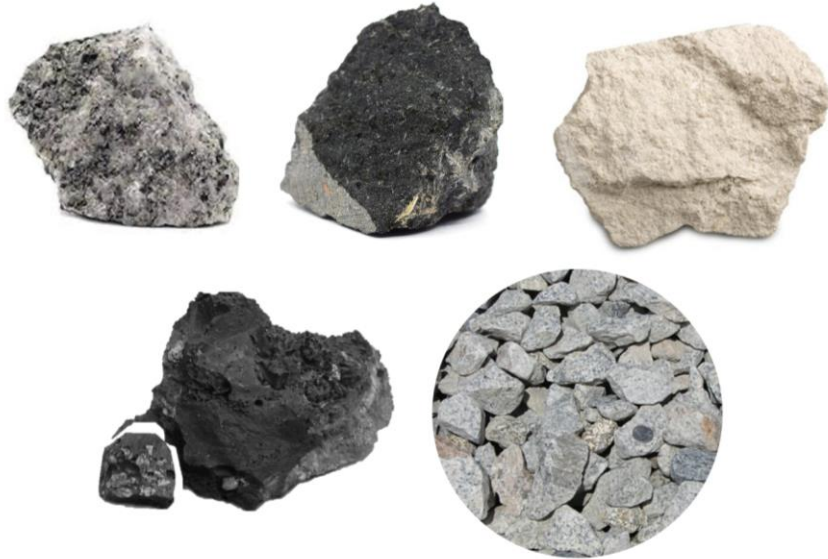
Figure 3. From left to right in the first row: Granite, Basalt and Limestone. From left to right in the second row: Slag and Gravel. (The constructor, 2019).
