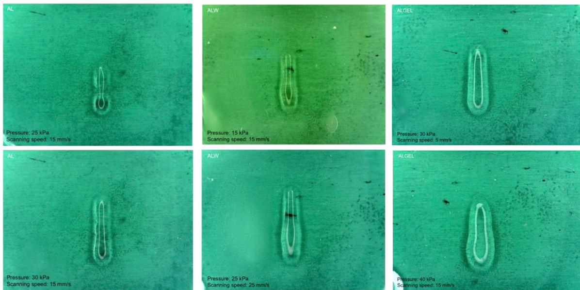
Figure 44 Photos obtained by the 3D printer chamber of the constructs printed at different pressure conditions and scanning speeds.
