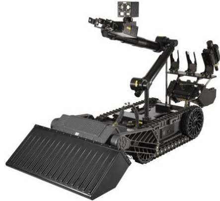
FIG 9 Mine-detecting robot for Korean AR operation
