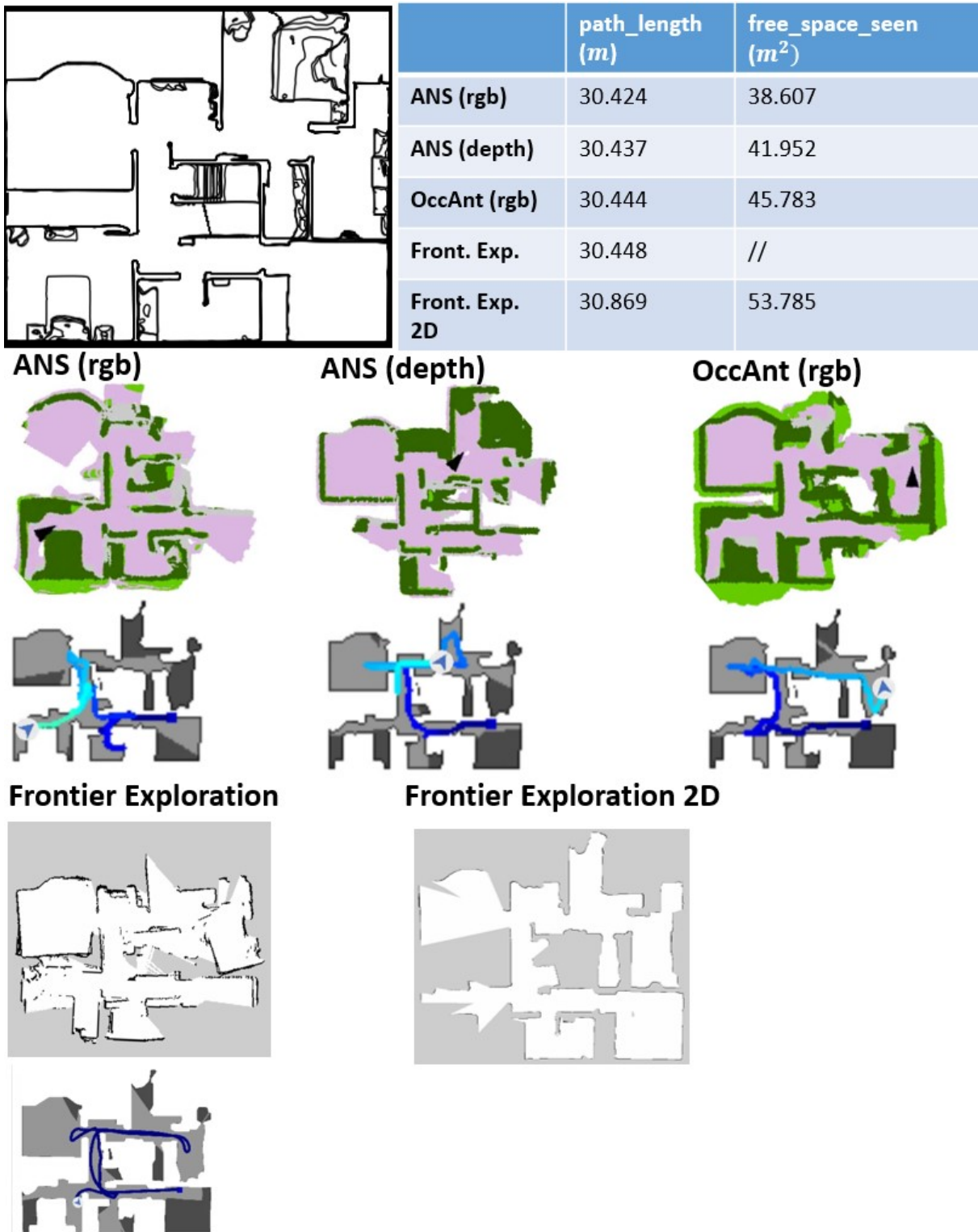
Figure 5.13: Map produced and path_length of ANS (rgb), ANS (depth), OccAnt (rgb), frontier exploration, and frontier exploration 2D in Scioto.
