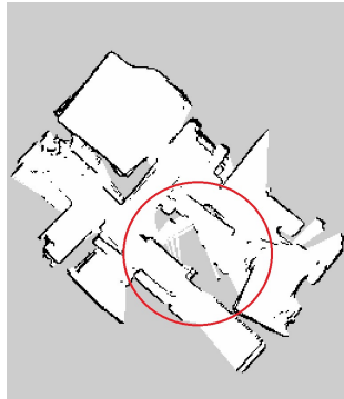
Figure 5.15: Example of incorrect laser readings in Scioto.
