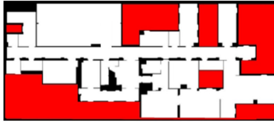
Figure 2.10: Example of map generated by [110]: in white the observed portions of the map, in red the unobserved portions inferred.
