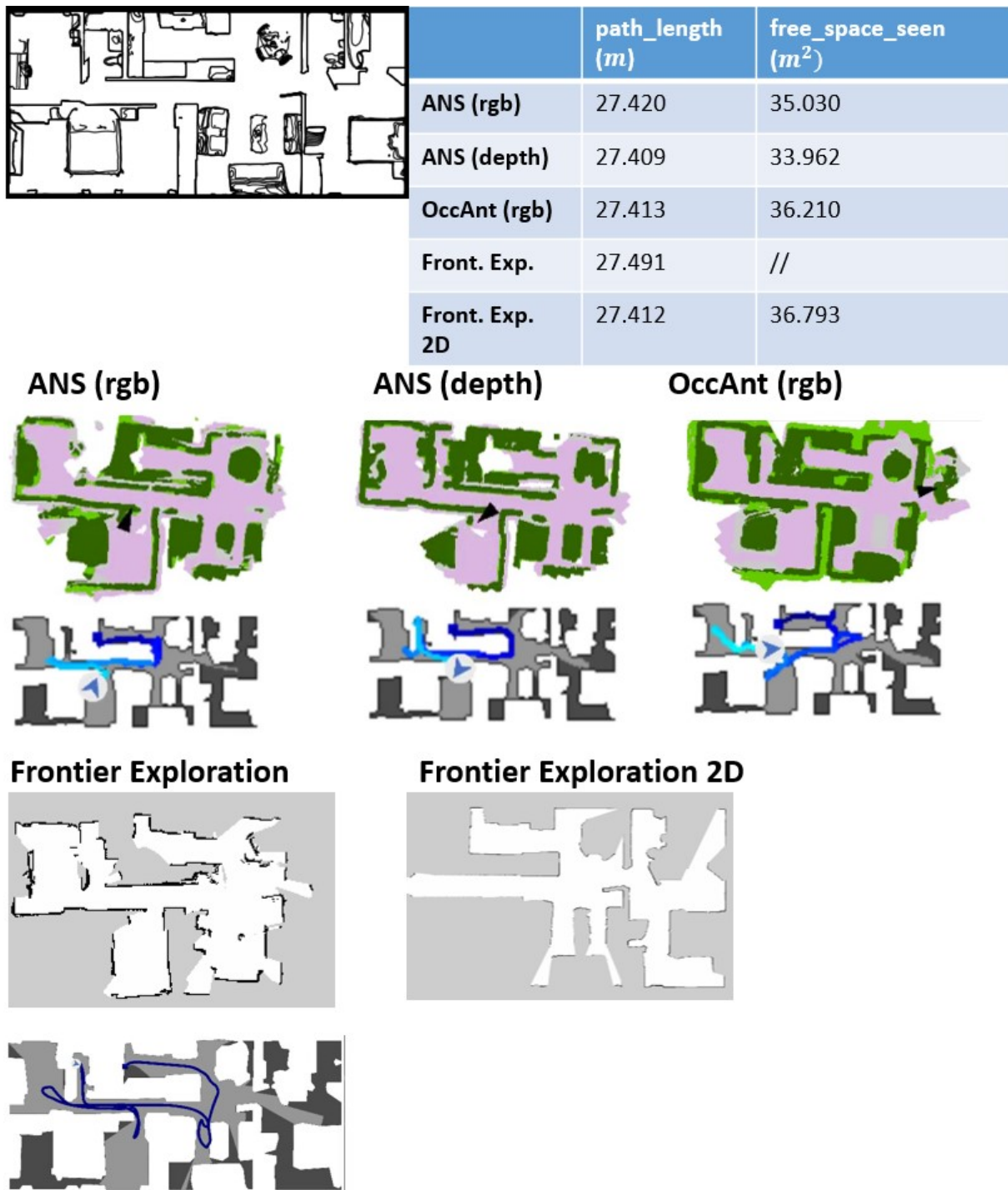
Figure 5.19: Map produced and path_length of ANS (rgb), ANS (depth), OccAnt (rgb), frontier exploration, and frontier exploration 2D in Cantwell.
