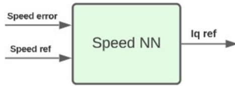
Figure 20: MLP Neural Network for the speed loop.
