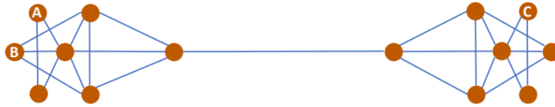
Figure 2.1: Positionally and structurally close nodes. Nodes A and B are positionally close, having relatively close positions in the global network. Nodes A and C are structurally close, having relatively similar local neighborhood structures. Courtesy of [6].
