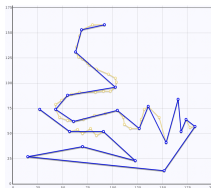
Figure 4.6: Simplification of the curve in yellow using the RDP algorithm with \epsilon=7,9
