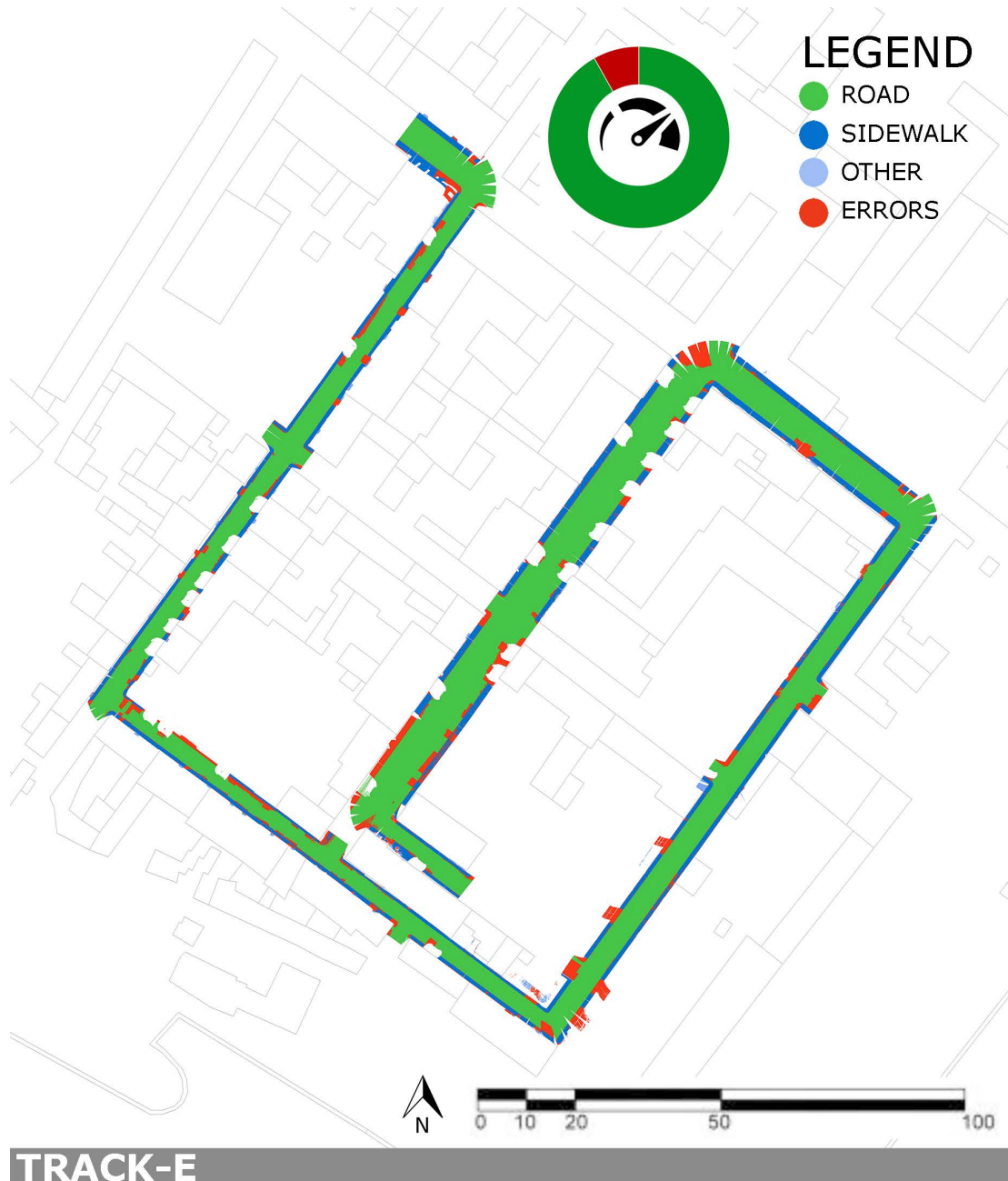
Figure A.24: Top view of the point cloud of Track-E after semantic segmentation with the knowledge-based method. Red points are errors. On the top part of the image, there is a pie chart with an overview of the whole points in the point cloud.
