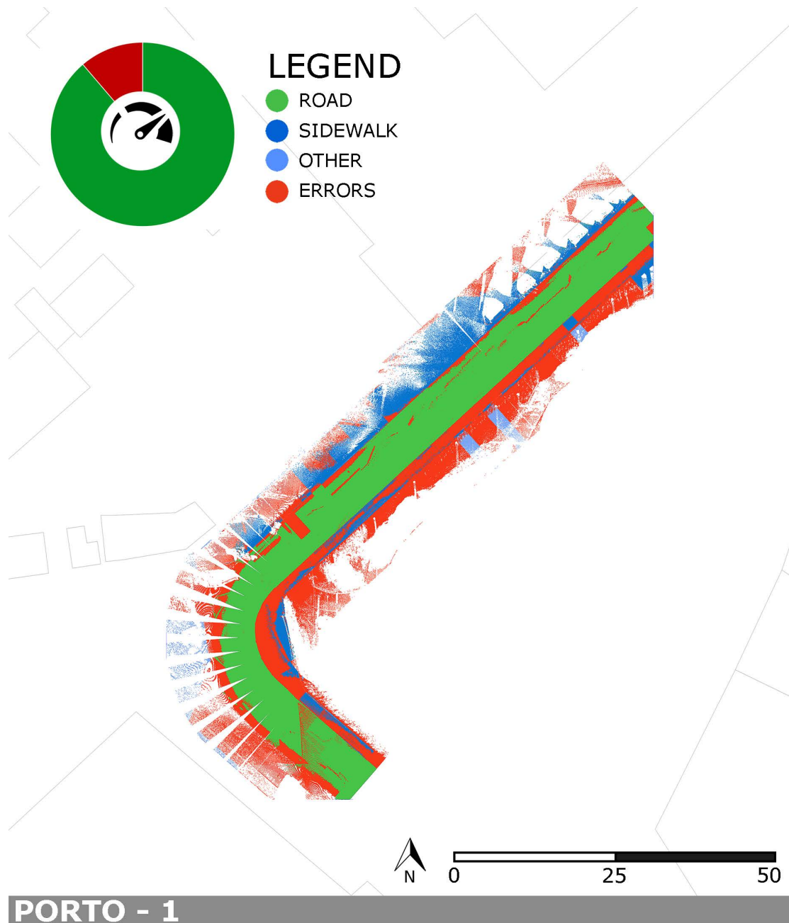
Figure A.59: Top view of the point cloud of Porto-1 after semantic segmentation with the knowledge-based method. Red points are errors. On the top part of the image, there is a pie chart with an overview of the whole points in the point cloud.
