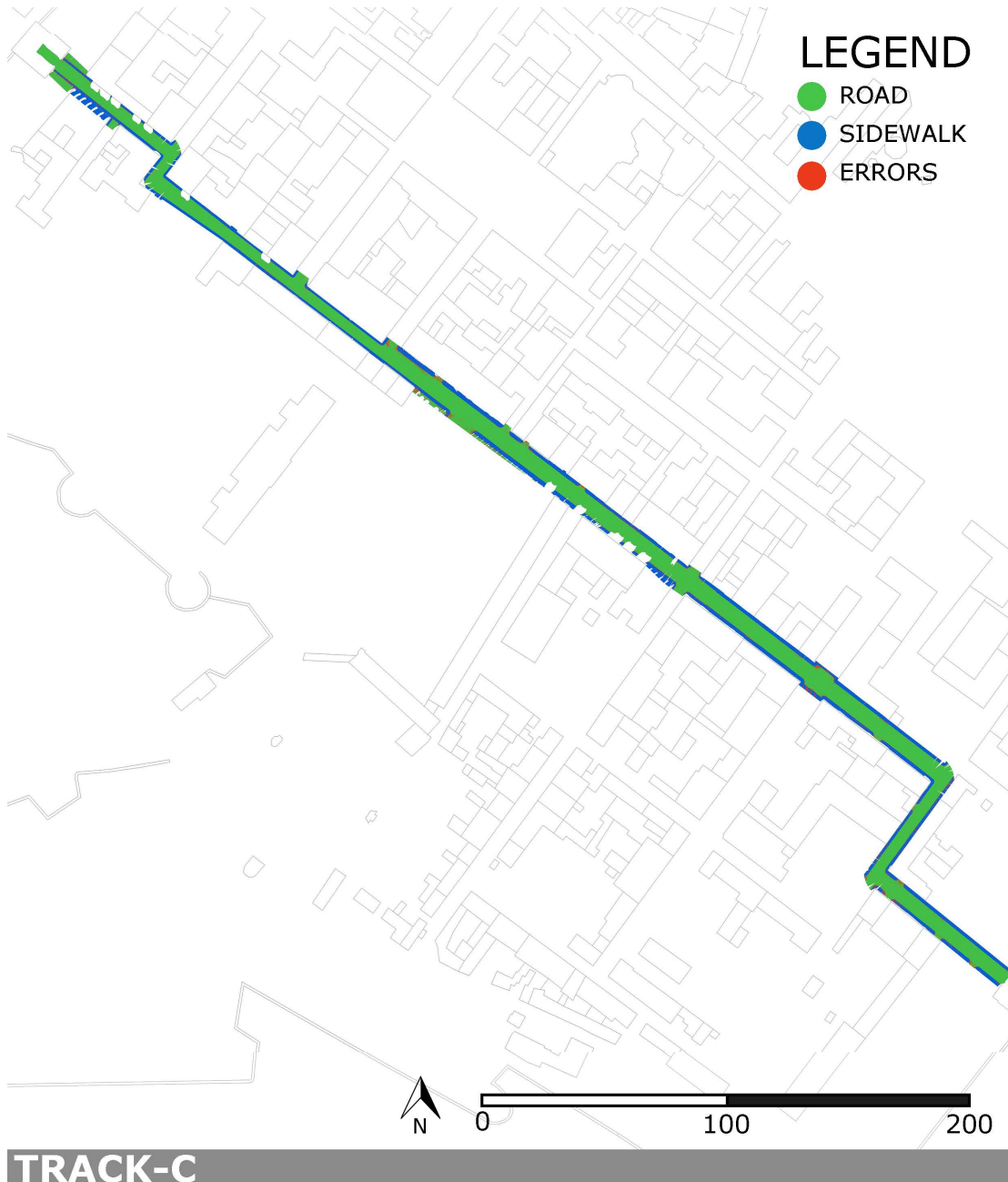
Figure A.15: Top view of the point cloud of Track-C after semantic segmentation with ML method. Red points are errors. On the top part of the image, there is a pie chart with an overview of the whole points in the point cloud.
