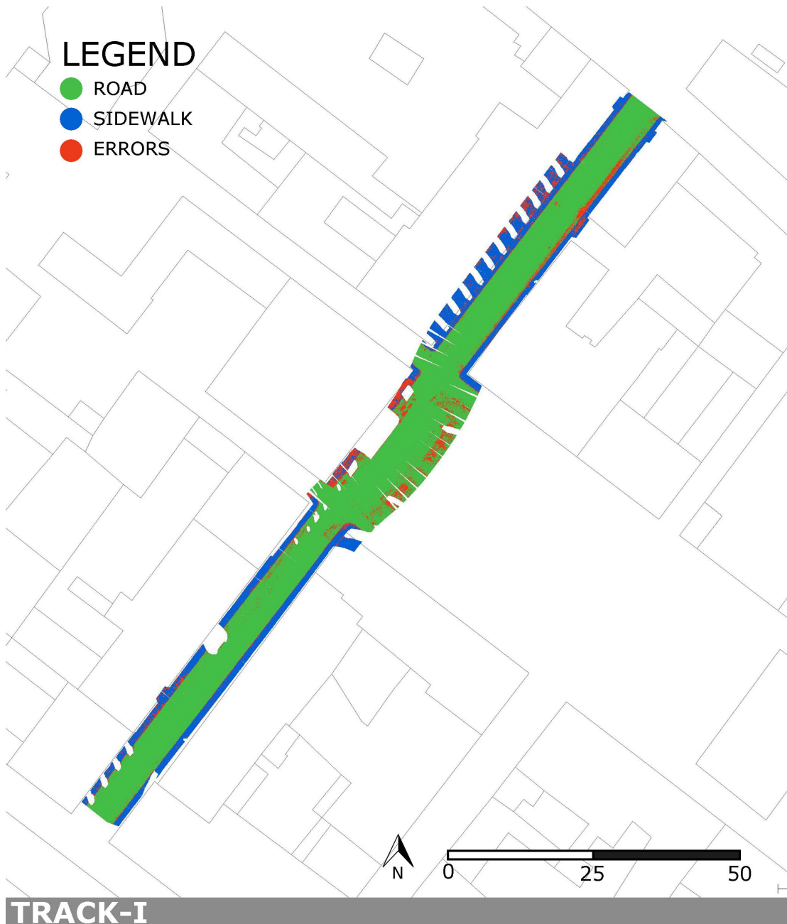
Figure A.40: Top view of the point cloud of Track-I after semantic segmentation with ML method. Red points are errors. On the top part of the image, there is a pie chart with an overview of the whole points in the point cloud.
