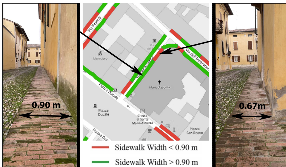
Figure 6.8: An example of direct comparison between computed and measured width. In the middle a portion of the sidewalk network with edges coloured according to the width if accessible ( >0.9\text{m} ) in green, or not accessible ( <0.9\text{m} ) in red. Comparing the results of the computation with the photos and measures taken on-site, it is possible to see the strengths of the method presented here.
