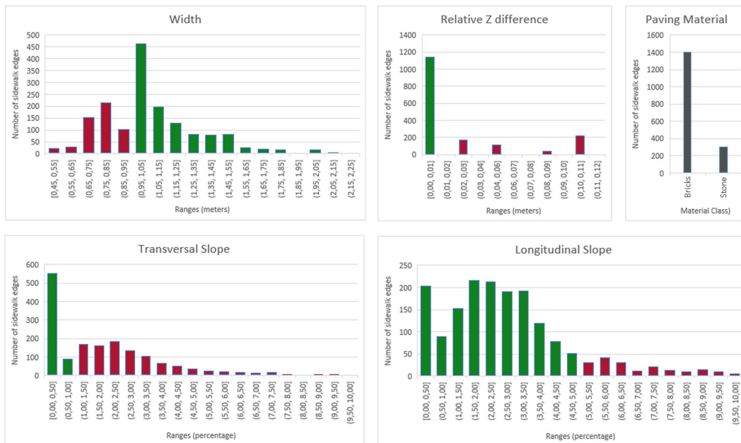
Figure 6.6: A series of bar charts representing the computed attributes and the distribution of their computed values. In red the values that respect the Italian reference, and in green the ones that do not respect the limit.
