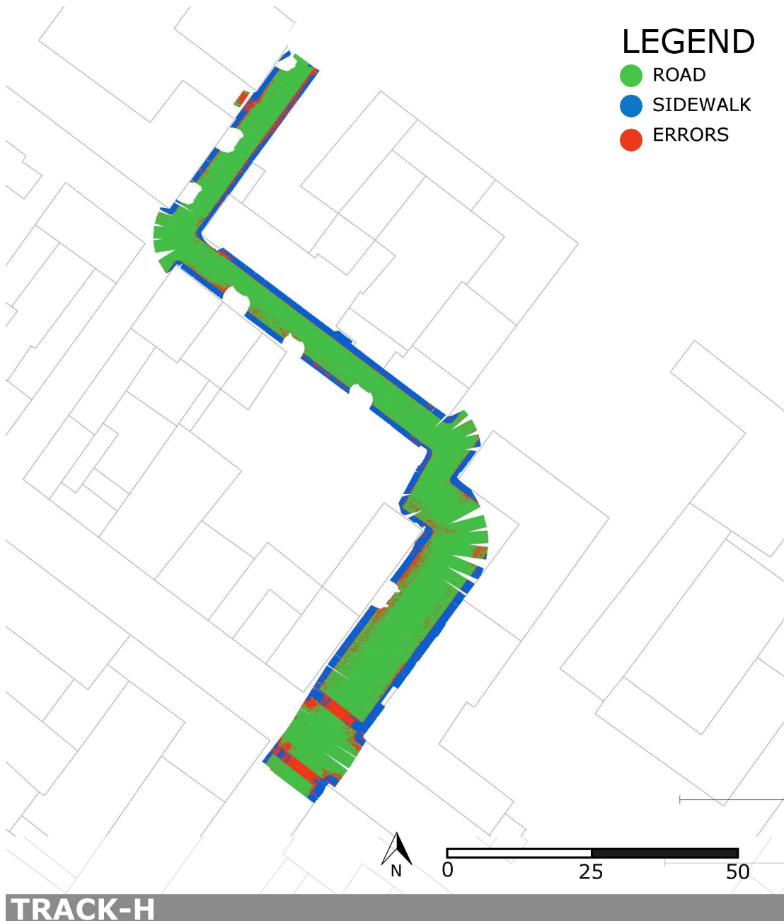
Figure A.35: Top view of the point cloud of Track-H after semantic segmentation with ML method. Red points are errors. On the top part of the image, there is a pie chart with an overview of the whole points in the point cloud.
