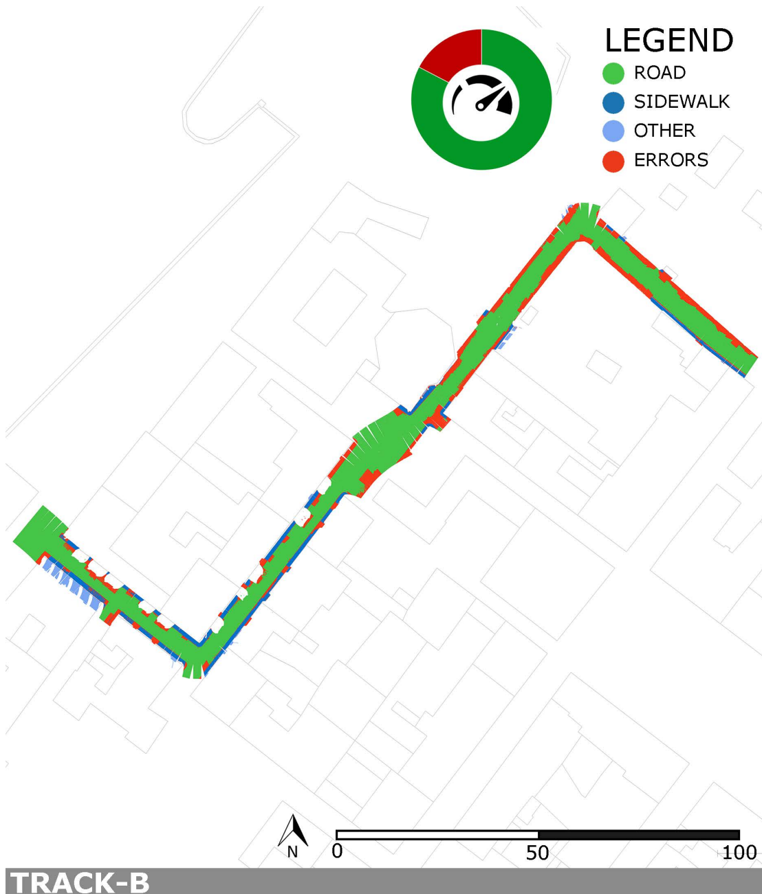
Figure A.10: Top view of the point cloud of Track-B after semantic segmentation with the knowledge-based method. Red points are errors. On the top part of the image, there is a pie chart with an overview of the whole points in the point cloud.
