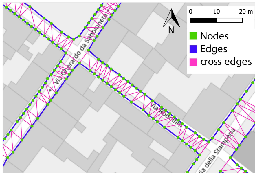
Figure 7.6: A portion of the city of Sabbioneta, green circles are the nodes, representing the sidewalks segments, blue lines are the edges connecting the sidewalks along the sidewalk path, and purple lines are edges that connects sidewalk nodes crossing the road, considering the possibility for a pedestrian to cross everywhere inside the historical centre of the city.
