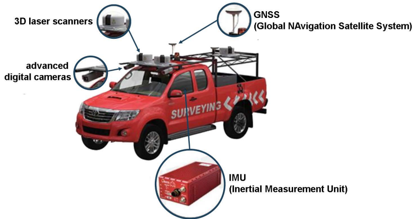
Figure 3.9: An exemplification of the instruments of a MMS mounted on a car.
