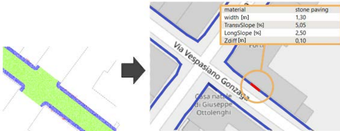
Figure 7.7: A screenshot of QGIS with the attributes of a selected edge highlighted, i.e. the attributes corresponding to the sidewalk segment identified by that specific edge.
