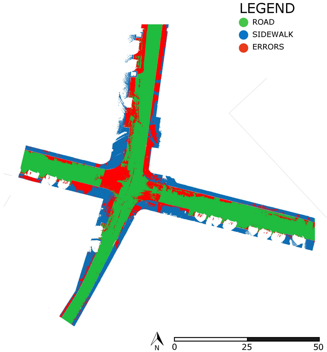
Figure A.67: Top view of the point cloud of Porto-2 after semantic segmentation with the ML method. Red points are errors. The training dataset was Track-C of Porto-2.
