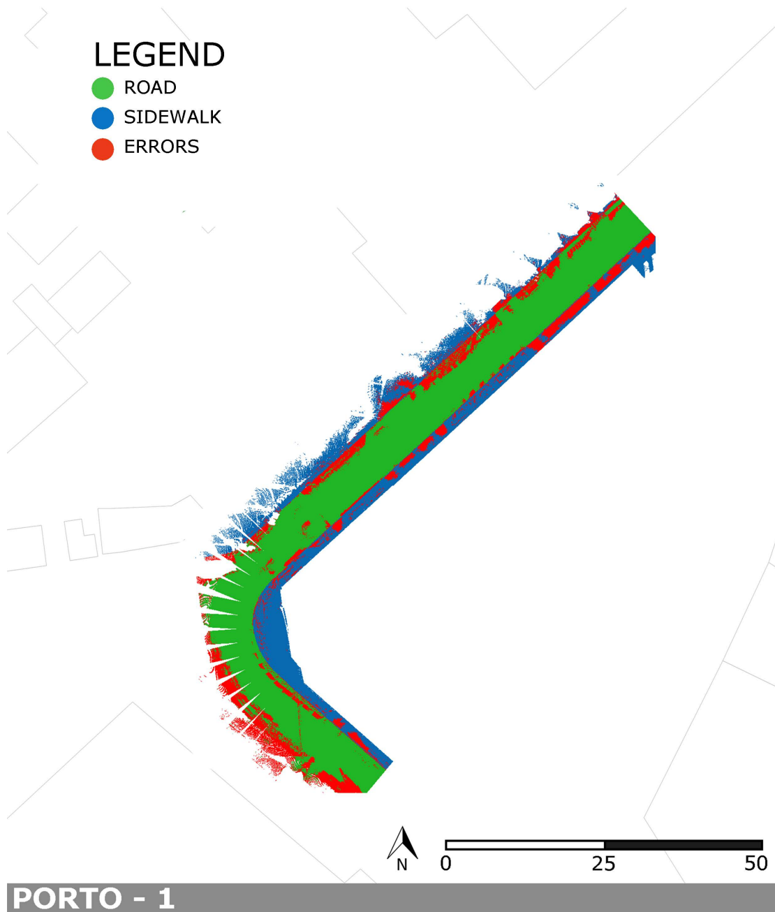
Figure A.60: Top view of the point cloud of Porto-1 after semantic segmentation with the ML method. Red points are errors. The training dataset was Track-C of Porto-1.
