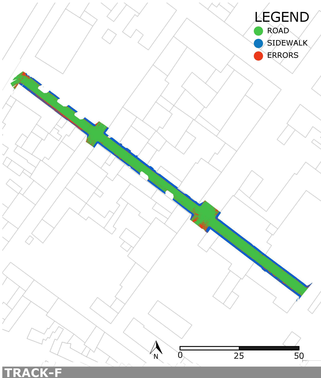
Figure A.30: Top view of the point cloud of Track-F after semantic segmentation with ML method. Red points are errors. On the top part of the image, there is a pie chart with an overview of the whole points in the point cloud.
