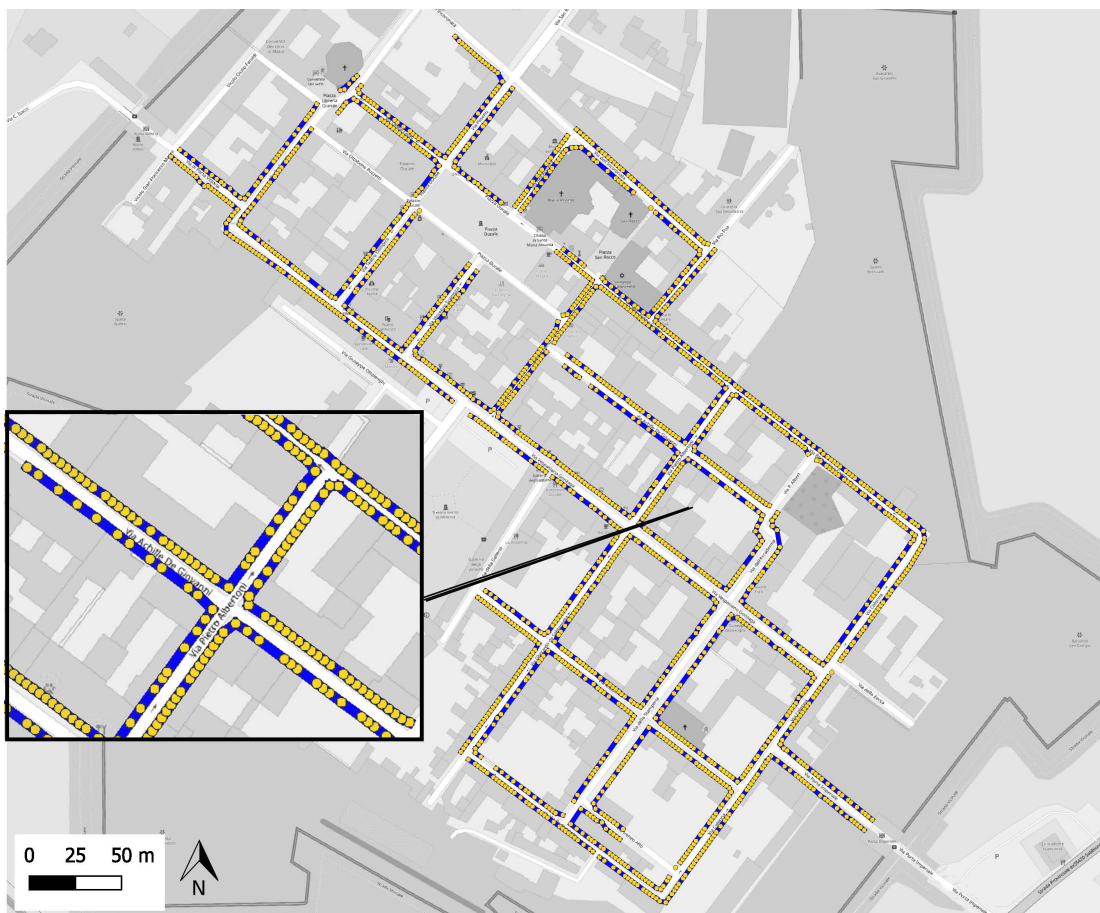
Figure 7.8: Result of the vectorization of the whole Sabbioneta dataset. In yellow the nodes and in blue the edges. A zoomed area helps to better see the results.
