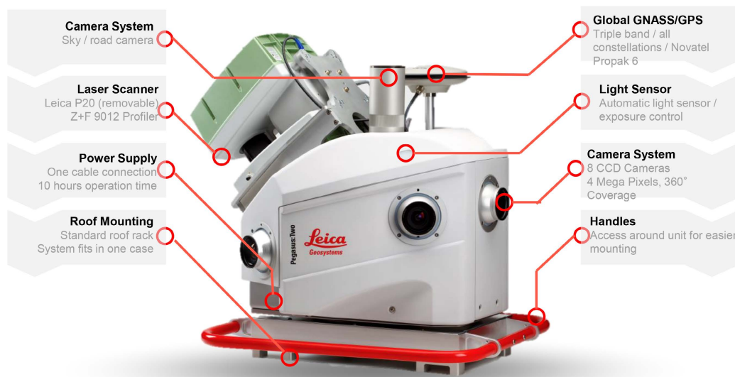
Figure 3.13: Leica Pegasus:Two and typically mounted sensors. From instrument's datasheet.
