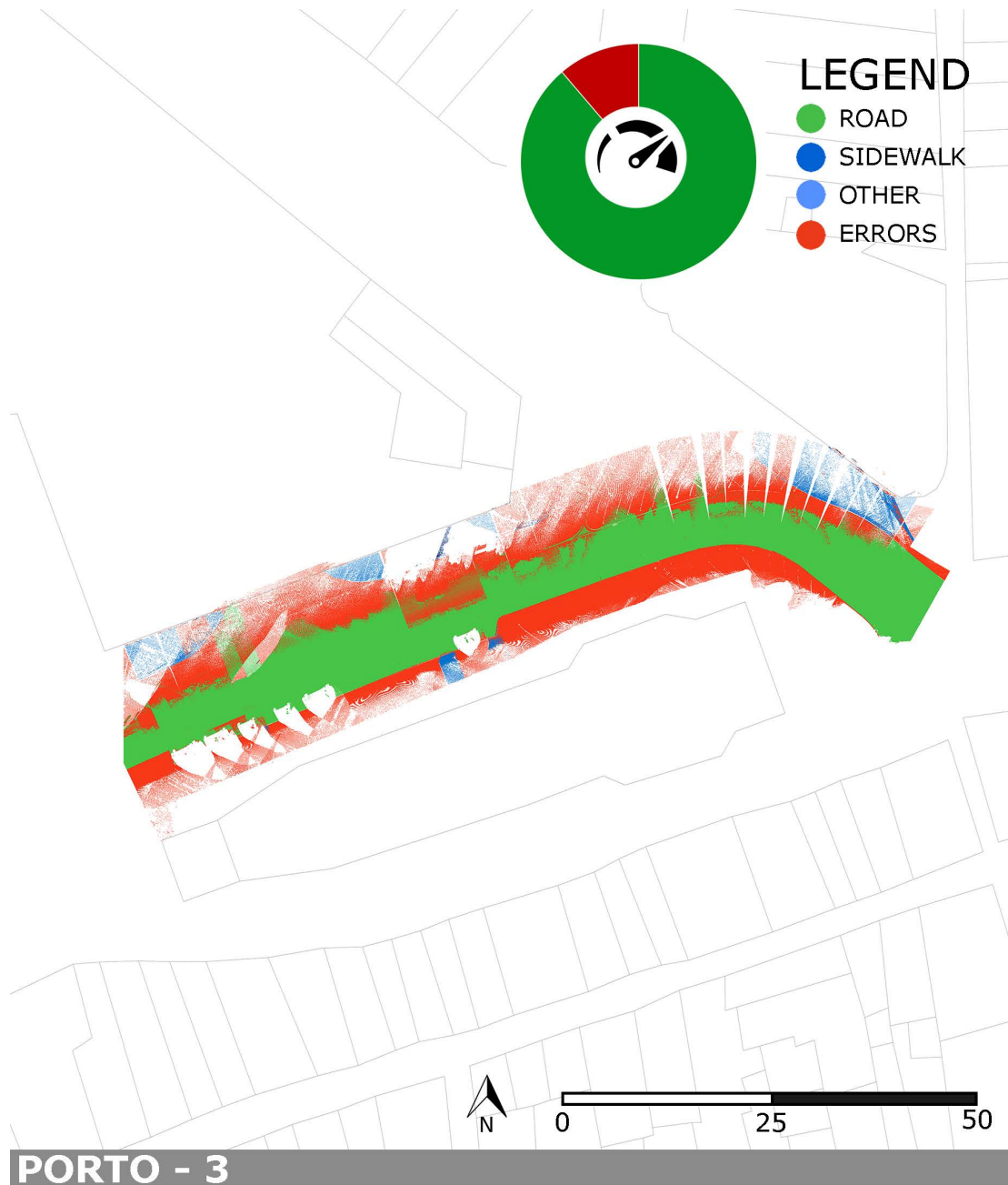
Figure A.73: Top view of the point cloud of Porto-3 after semantic segmentation with the knowledge-based method. Red points are errors. On the top part of the image, there is a pie chart with an overview of the whole points in the point cloud.
