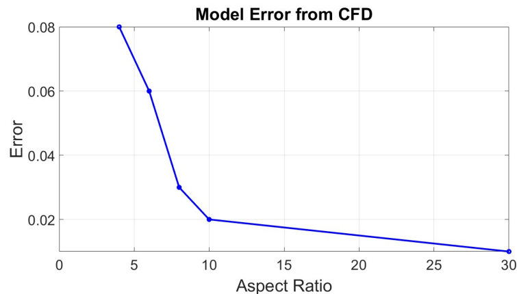
Figure 2.13: Error from CFD: variable height impact
