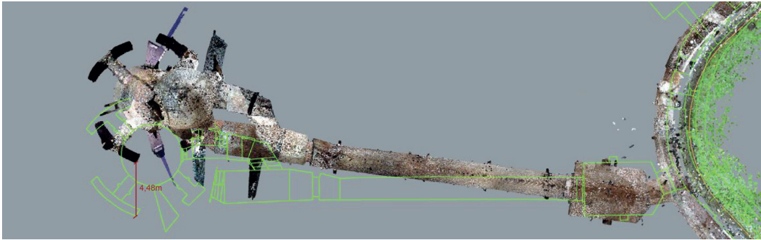
Figure 5.2.3.q Zoom of the point of maximum discrepancy between the 2002 survey and the point cloud.
