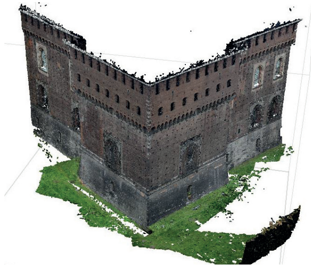
Figure 5.2.3.h Dense cloud obtained by photogrammetry of the facade of the Castello Sforzesco.
