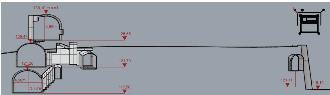
Figure 5.3.3.d Longitudinal section of the model of Torre della Colubrina (through the centre of the casemates).
