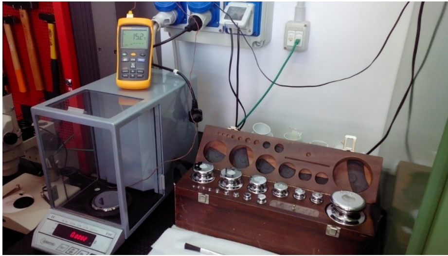
Fig. 4.2: overview of the set up to check the accuracy of the balance calibration
