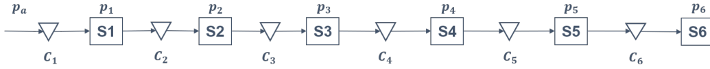
Figure 4.4: 6-station flow line used for the experiments in this work. Squares depict stations, while inter-operational buffers are represented as triangles.
