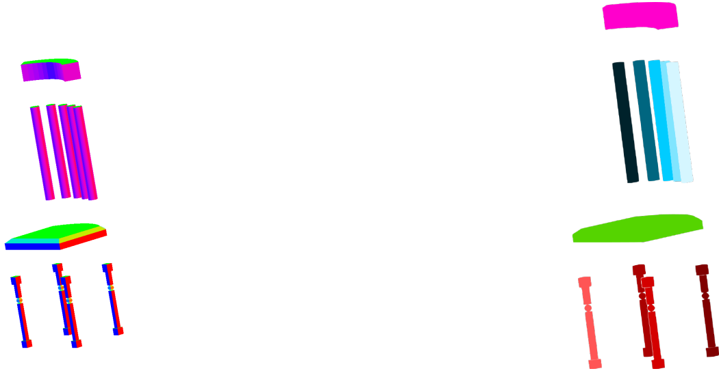
(a) The absolute value of the normals of the faces. Each component v_x, v_y, v_z of the vectors is represented respectively by the red, green and blue colour components
