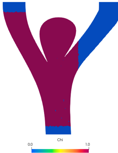
Figure 2.9: Representation of the the \chi function defined in 2D-Ane . \chi takes not null value around the bifurcation.
