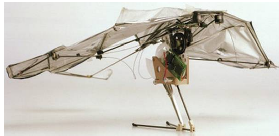
(b) Bioinspired jumping-gliding robot, Vidyasagar, 2015, EPFL [130]
