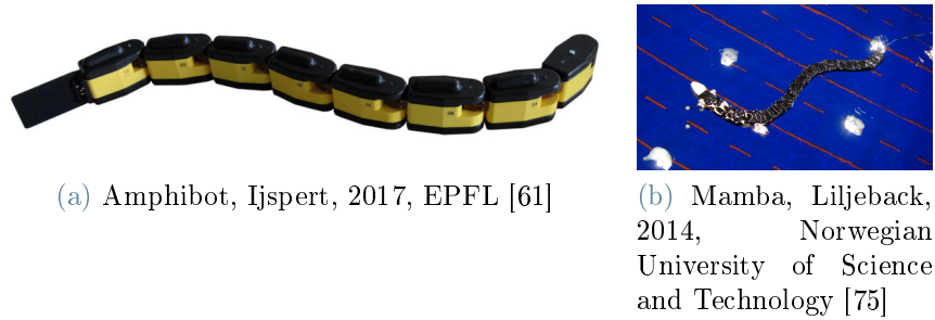
Figure 2.14: Robots inspired by anguilliform swimmers
