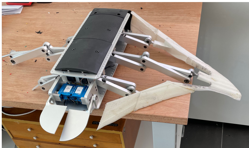
Figure 8.29: Structure of the fin mounted on the mechanisms
