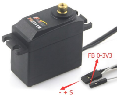
Figure 5.26: Feetech-FR5311M-360FB Continuous Rotation servomotor
