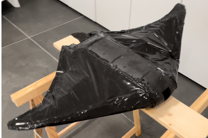
Figure 8.30: Robot with the fins made of silicone rubber sheets
