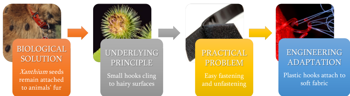
Figure 3: Scheme of the problem-driven approach with the invention of Velcro as an example
