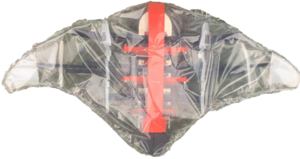
Figure 5.11: Assembled robot with coating
