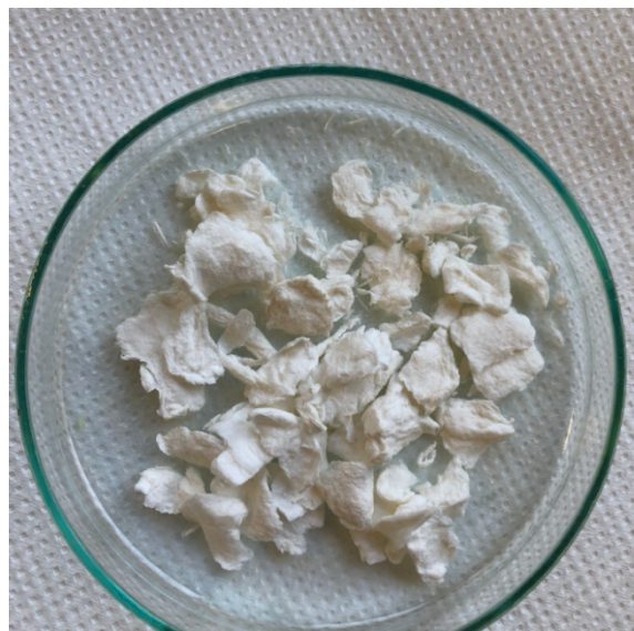
Figure 11. TEMPO-oxidized cellulose nanofibers from cotton linters
