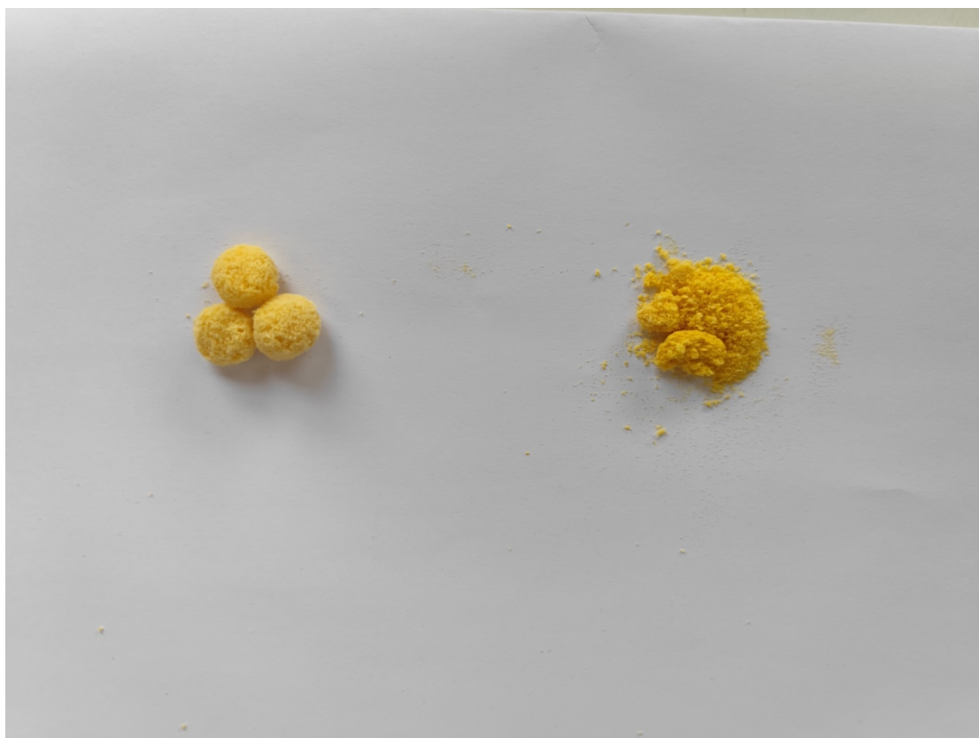
Figure 13. Comparison of CNS morphology prepared with different TOCNF: bPEI ratio, for 1:2 (left) and 1:1 (right)
