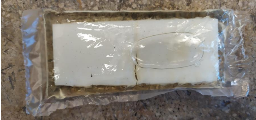
Figure 20: bag used to conduct creep tests in active environment
