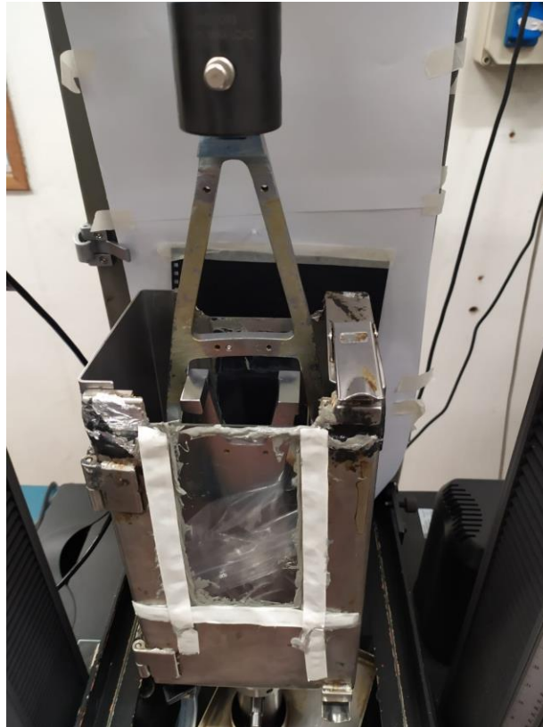
Figure 22: tank setup used for tests in active environment
