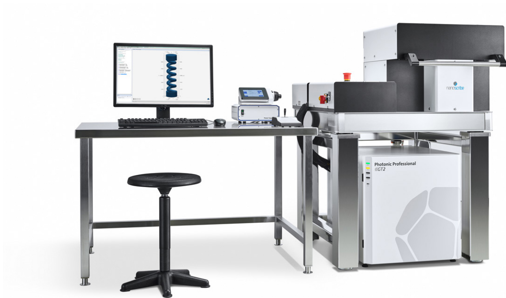
Figure 2.3: Photonic Professional GT2 setup used in this work: printer enclosure, control electronics, and workstation for job preparation and monitoring. Adapted from [36]
