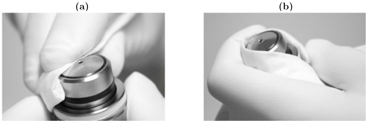
Figure 2.10: Objective cleaning procedure after GP-Silica printing. (a) Tissue-assisted cleaning around the lens by gently rotating the objective while keeping the tissue close to the lens center. (b) Wrapping the objective to collect solvent run-off during rinsing and prevent redeposition on the lens. Adapted from [37]
