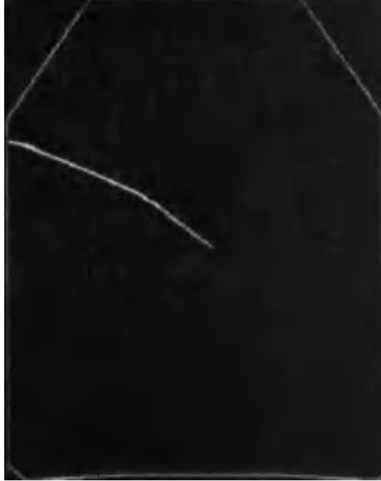
Figure 4.14: Radiography of a cracked ceramic layer of a SAPI [94]
