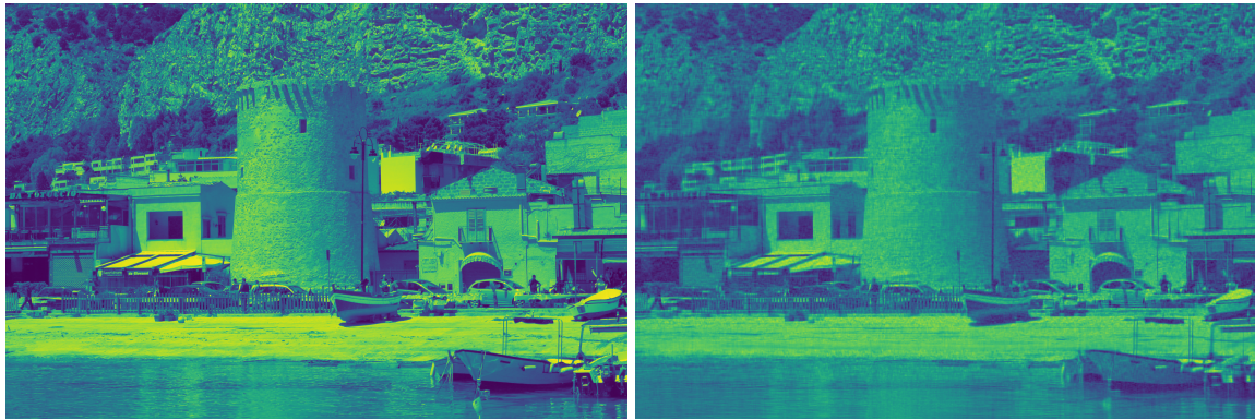
(a) 5184x3456 JPG image of Mondello (PA); red channel; standardized. Image size = 26,7 MB (b) Same image, retaining only the first 80 singular vectors-values. Image size = 17,4 MB
