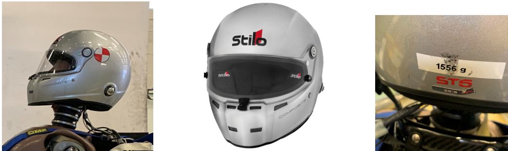
Figure 3.18: Helmet Stilo® ST5FN COMPOSITE
