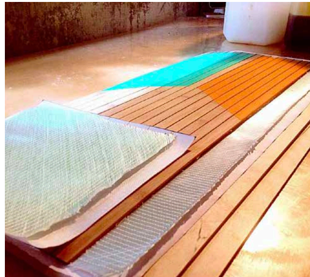
Figure 3.17. Different layers and materials I used to build a new deck, before the press
