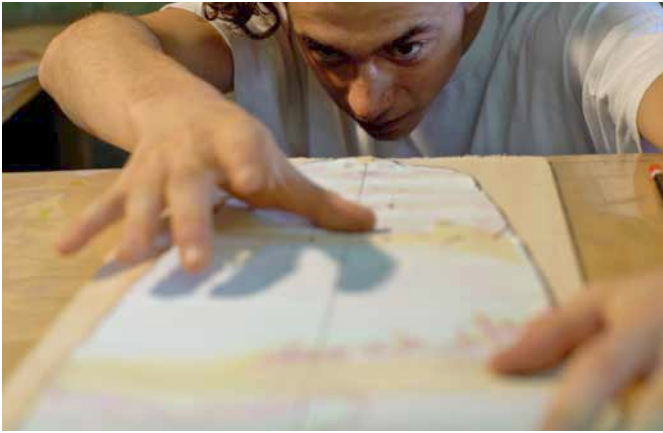
Picture 3.22/3.23. using a template to draw the board Picture 3.24. using epoxy resin to glue layers together
