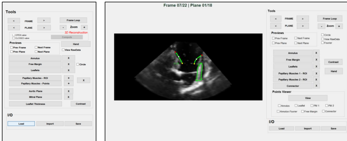
Figure 3.3: Left: menu of the starting GUI version. Right: new version of the GUI specially developed to allow a good segmentation of echocardiographic images of a TV. This version is the one that was used for manual image segmentation on this thesis work.
