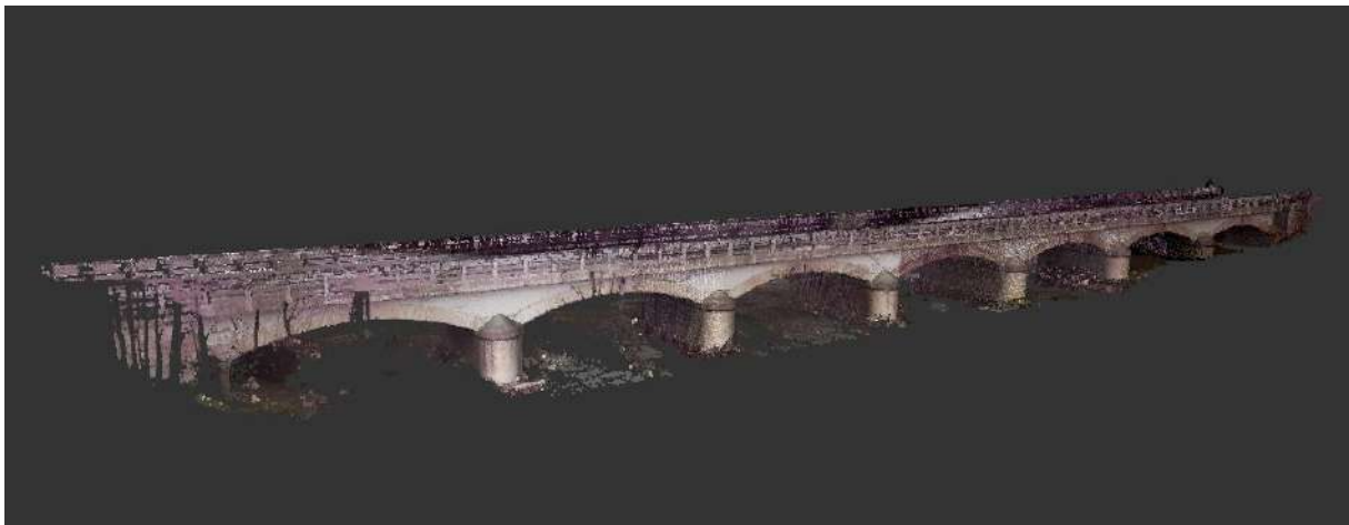
Figure 3.7: Point cloud by LiDAR data. Font: Autor.
