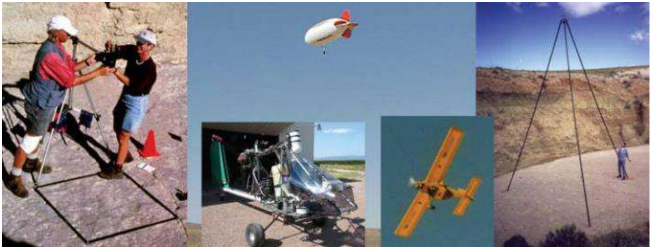
Figure 2.9: Variety of cameras and platforms used in close-range photogrammetry. Font: (Breithaupt et al., 2004)
