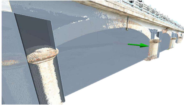
Figure 3.14: Visualization of automatic wall fitting. Font: Autor.
