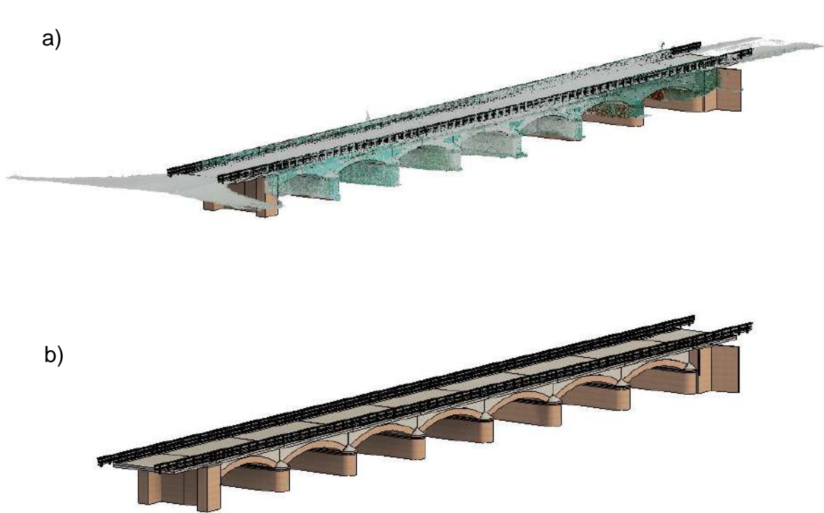
Figure 3.25: a) BIM model and point cloud data representation; b) only BIM model representation. Font: Autor.
