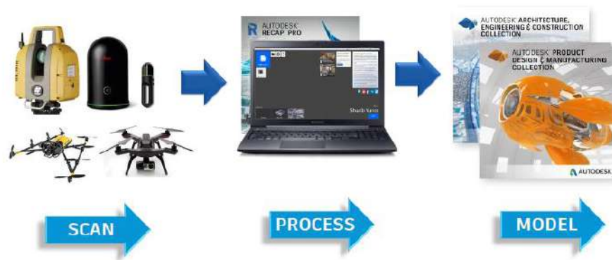
Figure 2.1: Standard scan-to-BIM workflow. Font: (Yunos, 2020).
