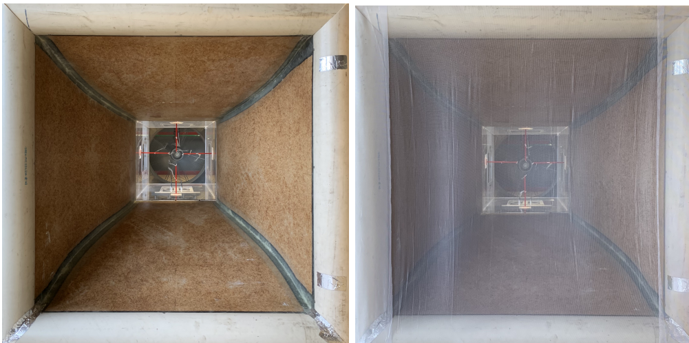
Figure 3.5: Flow visualization without (left) and with the honeycomb (right)
