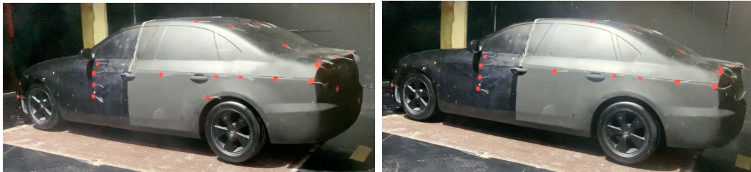
Figure 3.19: Flow visualization at a yaw angle of 0^\circ (left) and 10^\circ (right)
