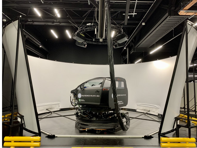
Figure 6.1: An overview of the DiM400 dynamic driving simulator
