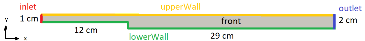
Figure 2.4. Geometry of our case, provided with dimensions and boundary names.
