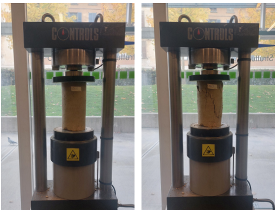
Fig. 9.39 - Before and after compression test for CW5
