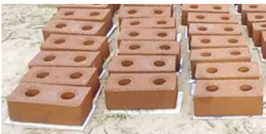
Fig. 6.11 - Earth blocks drying @Nairaland
