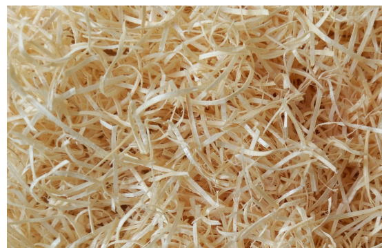
Fig. 8.41 - Wood fibers used in brick experiments
