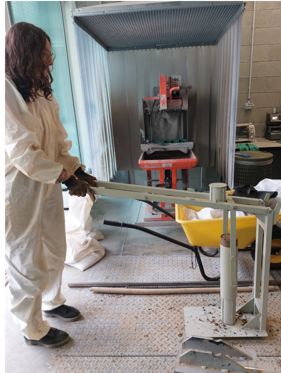
Fig. 9.22 - Step 4 : Compression of the raw earth
