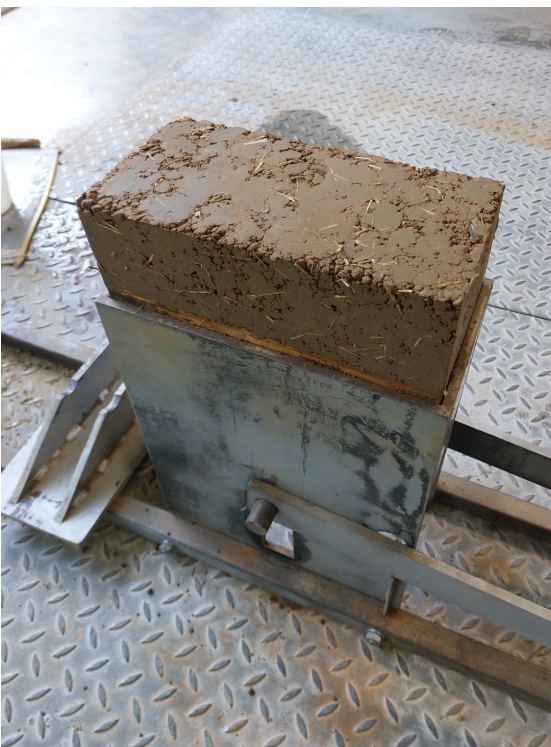
Fig. 9.23 - Step 4 : Extraction of the brick
