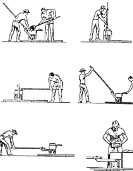
Fig. 6.10 - Operation of a CINVA RAM @G Minke
