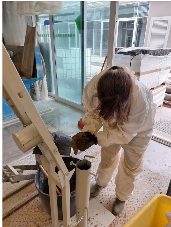
Fig. 9.20 - Step 3 : Filling of the cylinder press mould
