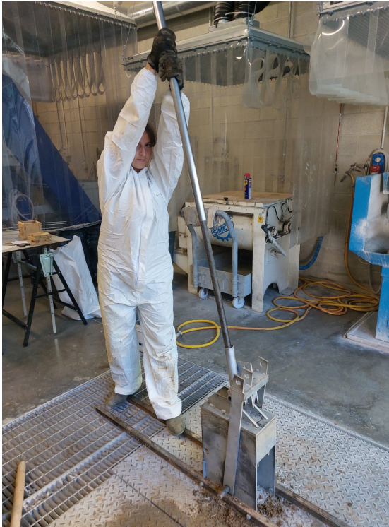
Fig. 9.21 - Step 4 : Compression of the raw earth
