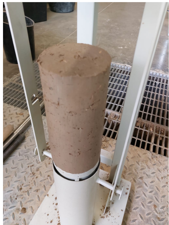
Fig. 9.24 - Step 4 : Extraction of the cylinder sample
