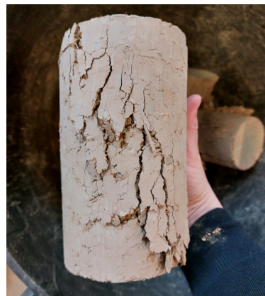
Fig. 9.30 - Diagonal and parallel cracks for CB1
