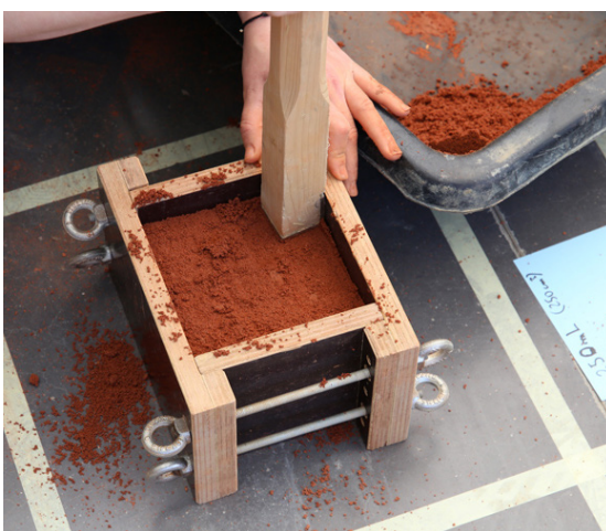
Fig. 3.13 - Humid soil sample compressed @AMACO
