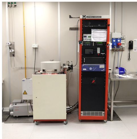
Figure 2.4: Picture of the Leybold LH Z400 magnetron sputtering system in Polifab's deposition area.
