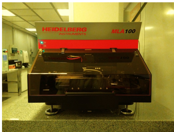
Figure 2.2: Picture of the MLA100 maskless aligner in Polifab’s yellow room.
