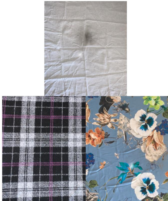
Figure 66: The three different fabrics used in the experiments; (top) cotton, (down left) wool and (down right) polyester.
