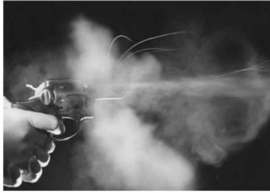
Figure 22: The plume of gases that escapes a weapon, in this case a revolver, when it is fired [5].
