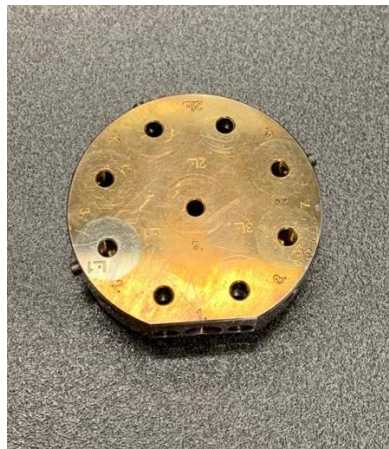
Figure 79: The stub holder of the SEM; it can receive till 9 stubs.
