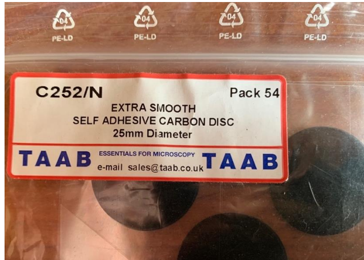
Figure 76: The adhesive layer coated with carbon used on the aluminum stubs to collect the GSR.
