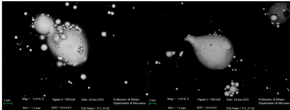
Figure 101: Two examples of particles that derive from a bigger one. In the left image there is a smaller particle that is detaching from the bigger core while in the right image there is a particle that seems a droplet with a broken bridge which probably comes from a bigger core from which this particle has detached; these particles are collected from the polyester.
