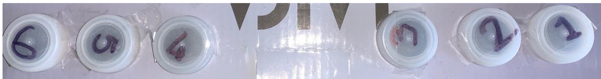
Figure 77: Stubs handling arrangement; each stub is inserted in the cardboard, covered with a cap and fixed with a scotch; in this figure, the first six stubs are showed. .
