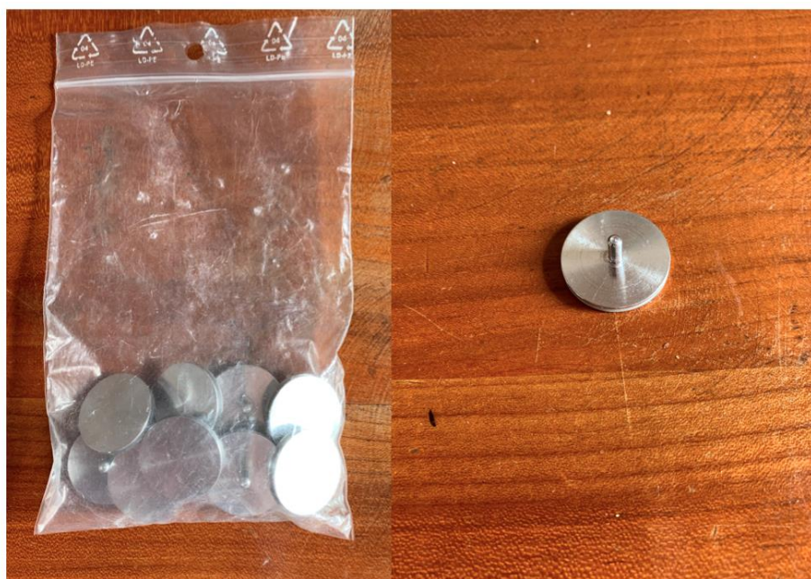
Figure 75: Aluminum SEM's stubs used to collect GSR.
