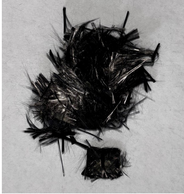
Figure 3.4: Dry fibres obtained from the matrix digestion test.
