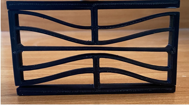
(a) Deformation of 3D printed Nylon NS honeycomb cell, under compression
