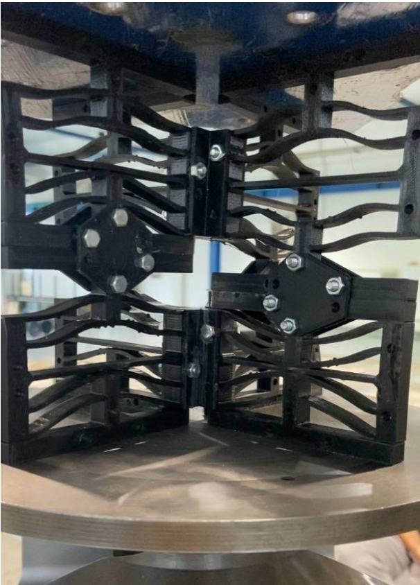
(c) Stage III - Second Snap-Through event
