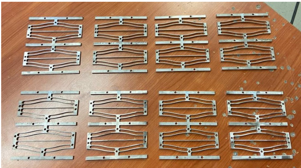
Figure 2.33: Picture of the Negative Stiffness Honeycomb third iteration modules before assembly
