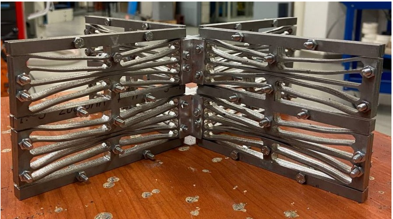
Figure 3.31: Third iteration model after the second dynamic compression test
