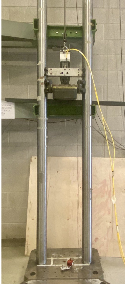
Figure 2.23: Vertical sled used to perform dynamic compression tests
