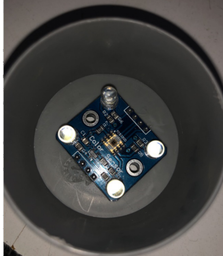
Figure 3.10: Color Sensor Embedded in a Cylindrical Cover Structure.
