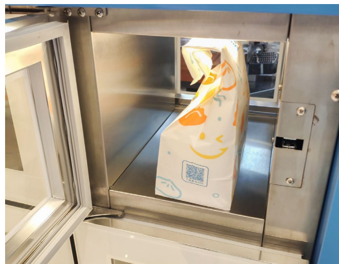
Image 3.8 The self-pickup cabinet has a two-way window, so consumers do not have to have direct contact with staff
