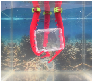
Figure 10: Grasping execution phase during the pinching of the plastic box.
