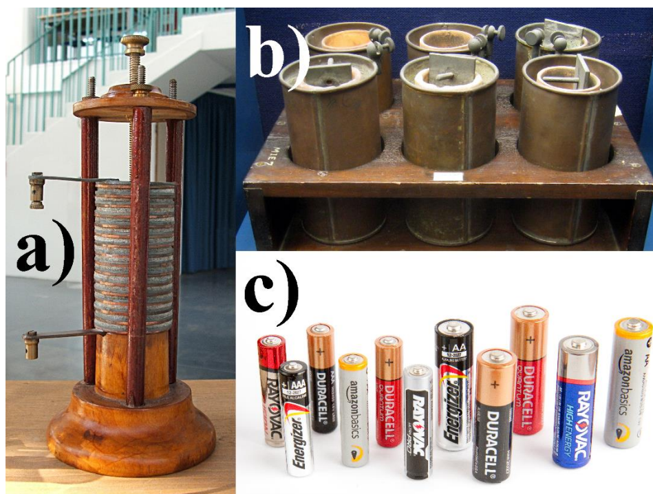
Figure 10 – Different primary batteries. a) Volta pile b) Daniel cell c) alkaline batteries.
