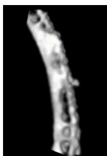
Figure 41- A thin section of the deposit on the inner rod of the cell without additive after the second cycle. It is visible that in this area the new deposit formed a crust above the previous layer, leaving a cavity in between.
