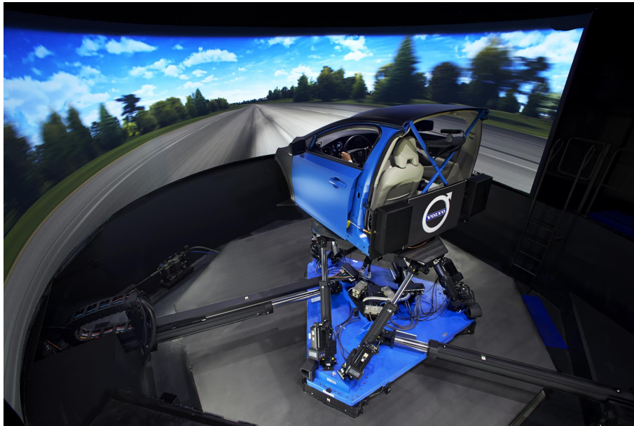
Figure 7.21: Dynamic driving simulator DiM 150 at Volvo Cars (Source: Volvo Cars database).
