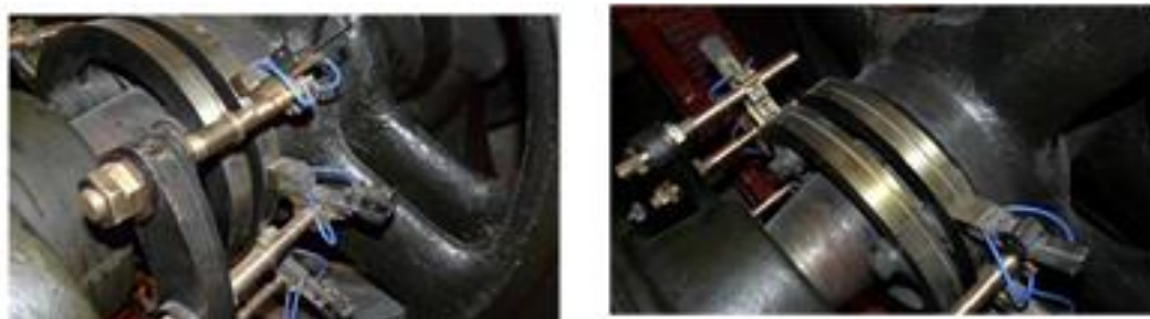
Figure 4.16: Stationary brushes and ring collectors
