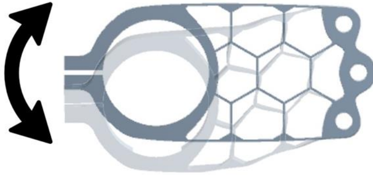
Figure 34. Mode shape named by the author as lateral bending.
