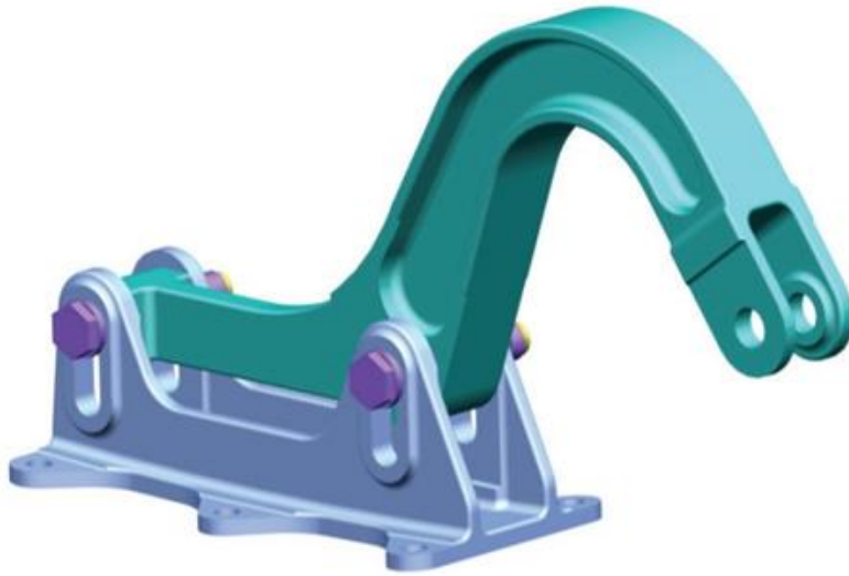
Figure 16. Initial model to be optimized. In green is the piece subject to the topology optimization analysis.
