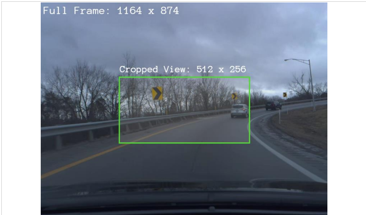
Figure 17 - Comparison between the cropped frame and the full-frame acquired by the device's camera
