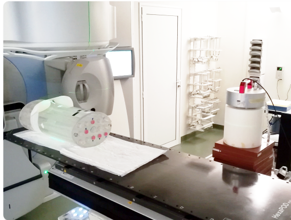
Figure 3.2. BOMAB phantom with silicon breast. At the right, the LUPIN detector
