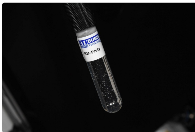
Figure 2.7. A bubble detector personal neutron dosimeter
