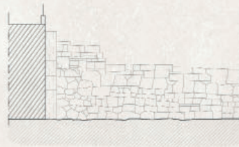
phase 1 existing walls leading from the first phase of excavations in the 1980s. These walls appear as historical stone masonry but, although visibly evident, were built with similar material to the new ones
