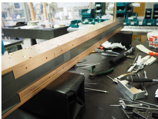
(a) TCPPM jaw with MoGr blocks installed.
