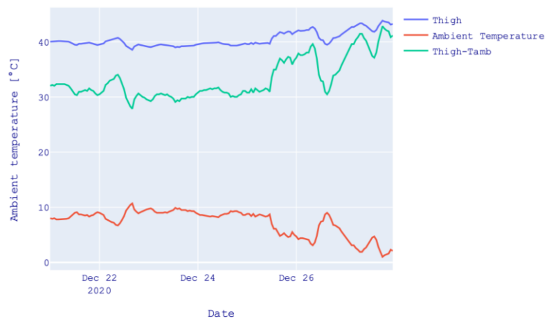
Figure 40: Temperature variation in time for AW/W hp floor.
