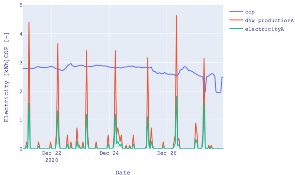
Figure 57: DHW production vs HP electric consumptions vs HP COP for Configuration n.4.
