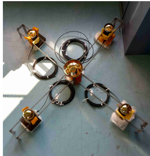
Figure 8: Holding test of cross holder using the 5 PMTs of the reference configuration (before reinforcement of the cross arms).
