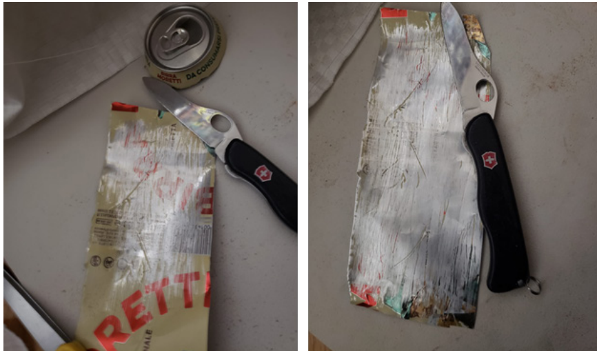
Figure 33: Shows the progress in scraping off the paint of the aluminum cans with a blade
