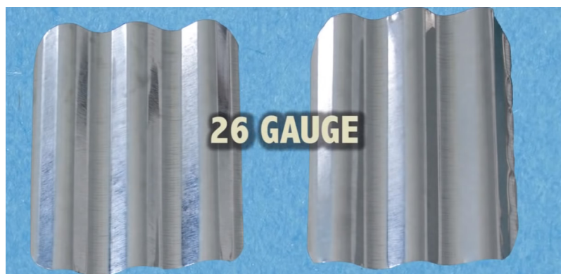
Figure 42: Shows the Galvanized Steel Sheet used for the Solar Bottle Bulb, as roof support
