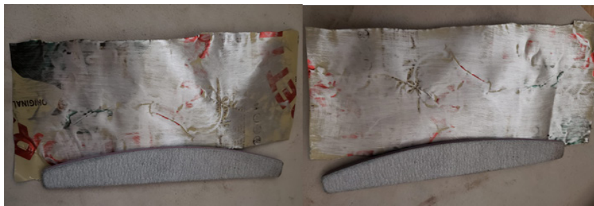
Figure 34: Shows the progress in scraping off the paint of the aluminum cans with a sandpaper
