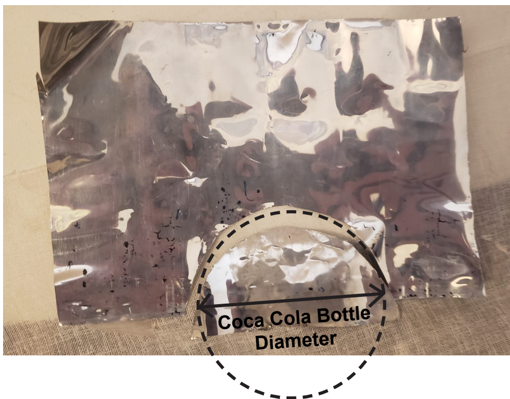
Figure 38: Shows the method to create a halfcircle in the aluminum sheet to be then used as material for the parabola
