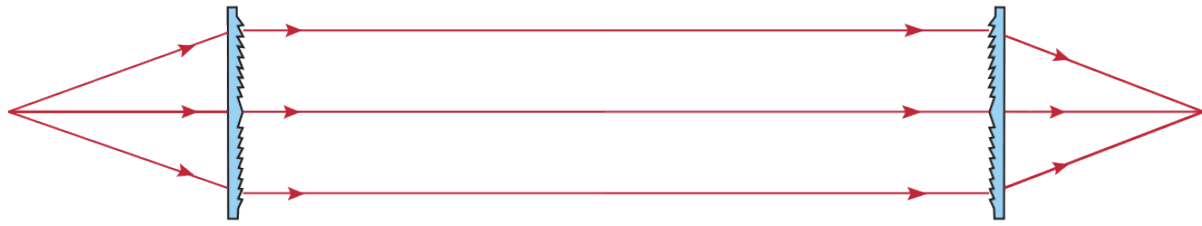
Figure 23: Light Collimation of a point source with a Fresnel Lens
