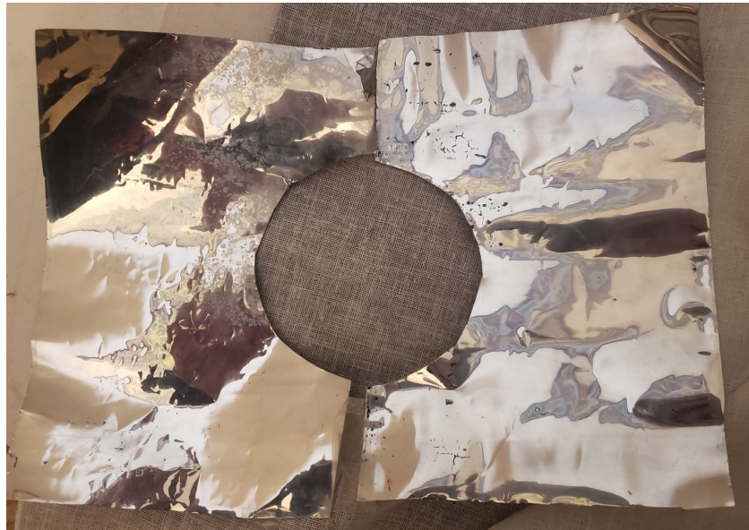
Figure 39: Shows the method to create the parabola by joining the two aluminum sheets, with the cemicircle perviously cut
