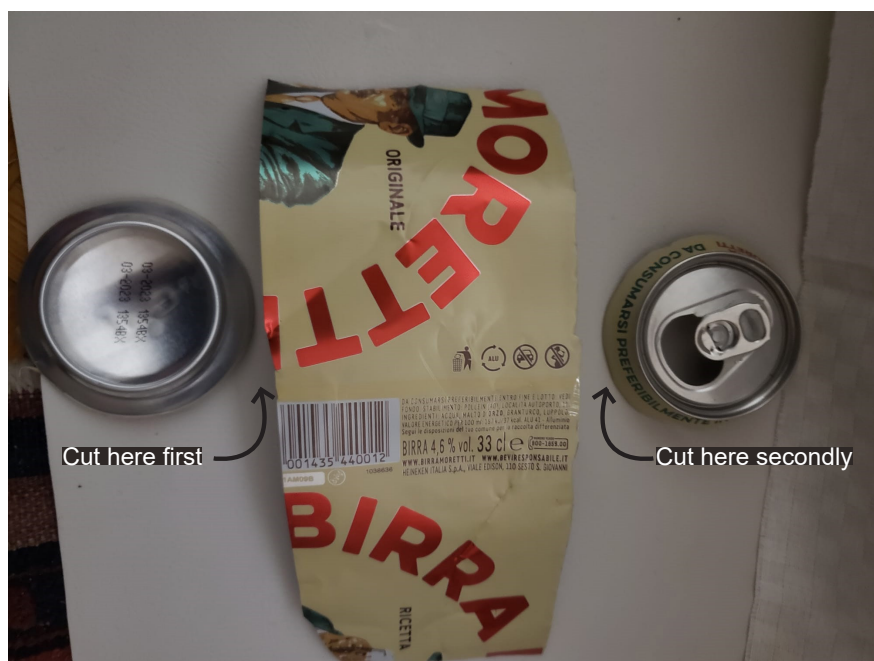
Figure 32: Shows where the aluminium can needs to be cut
