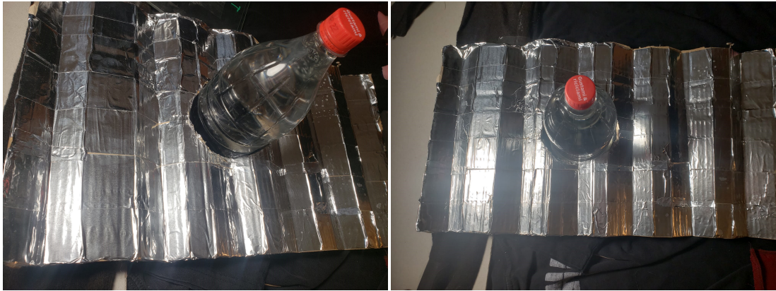
Figure 43: Shows the simulated Galvanized steel roof sheet used in Test 2.3
