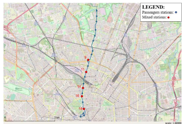
Figure 4: Disposition of mixed stations along Line 4
